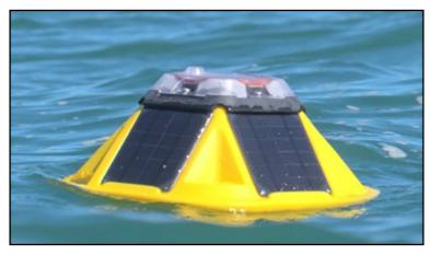
Wave sensor buoy
